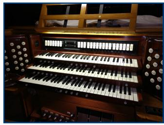
Also included in this stage was the restoration of the Choir division and the smaller Pedal stops (16' Bourdon, 8' Flute, 8' Violoncello). The pipes were brought to our shop for cleaning and repairs, then adjusted for evenness of speech and tone. The ventil-style Pedal windchests were releathered and fitted with new primary magnets.
